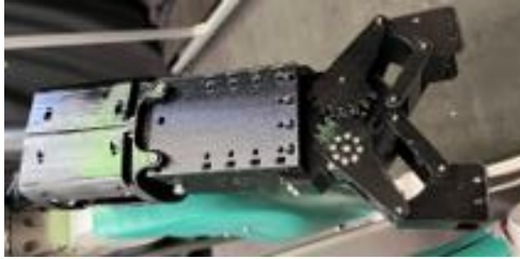
Figure 4: Bimanual “lobster claw” gripper installed onto Digit forearm.
